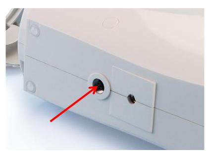
Modified data are transferred to the RCS instrument by using serial RS232 interface
